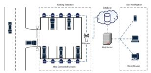
Fig. 1 Typical system model for smart parking system
